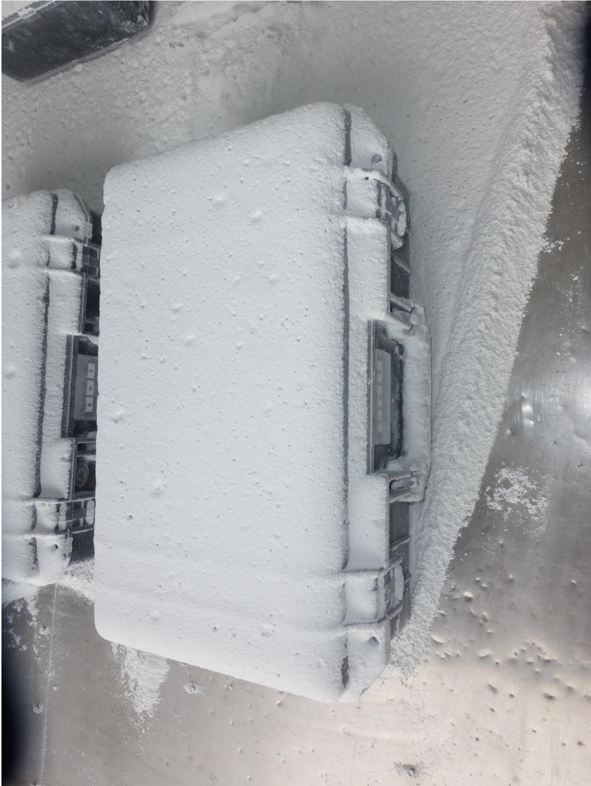
Photograph 4 Dust - Post Test
