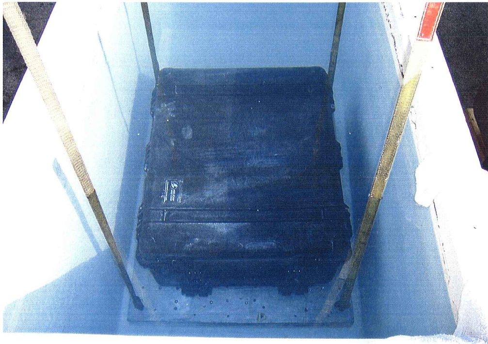
Photograph 3 Immersion Test Setup
