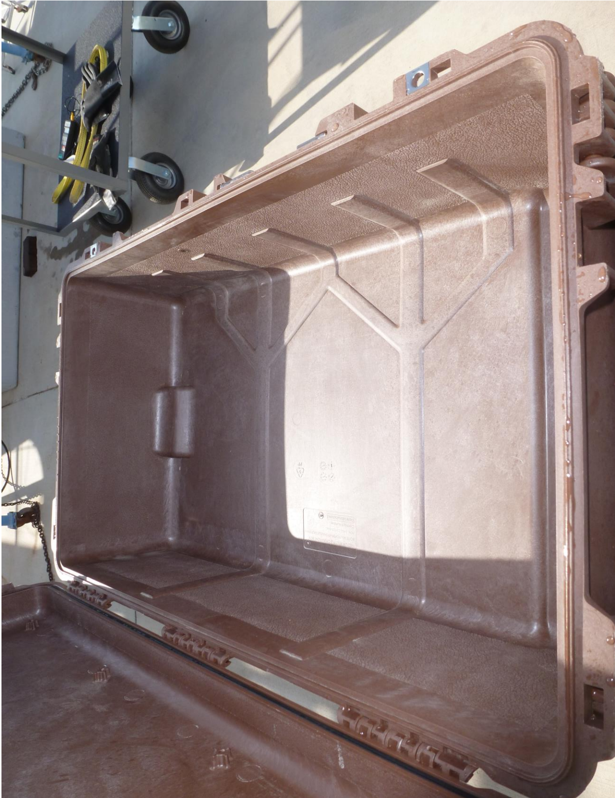
Photograph 12 Leak Test - Immersion - Post Inspection
