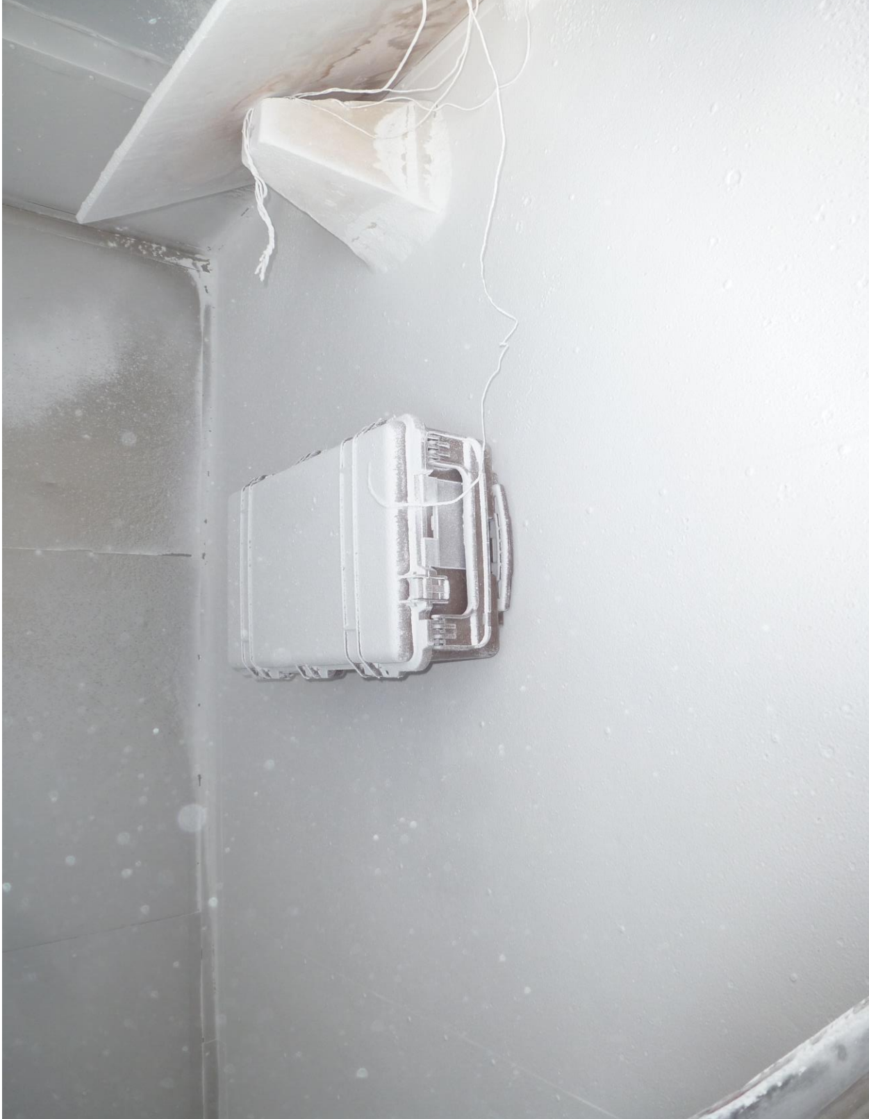
Photograph 14 Dust IP6X – Post Test
